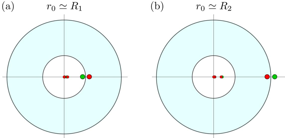
Figure R.3: When the vortex gets close to the inner (a) or outer (b) boundary, the dominant effect is the interaction with the closest image with opposite sign. This results in opposite signs for the angular velocity of the uniform precession.
