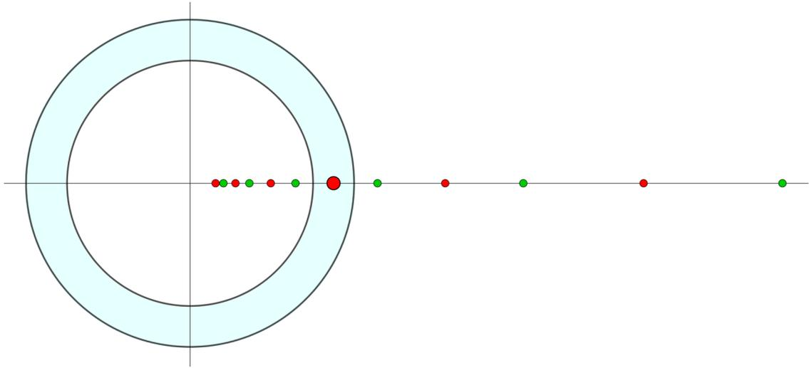
Figure R.1: Schematic representation of the infinite set of image vortices required in the annular geometry. The first pairs for  $m \in [-3, 2]$  are explicitly shown. The positive physical vortex is the red dot inside the blue shaded area and it has a bigger size for sake of visibility. The color of the dots is associated to the charge of each vortex that can be either +1 (red) or -1 (green). Only the closest image vortices are shown, beyond both boundaries.
